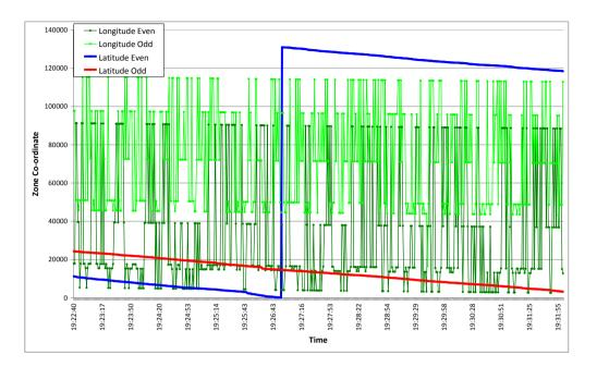
2.2 The data shows that even prior to decoding the aircraft position the encoded values for longitude exhibited multiple jumps. Normally these values should follow a saw tooth pattern with jumps corresponding to when the aircraft position crosses a zone boundary as shown below :
