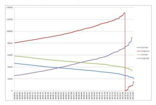
2.3 The continuous jumping pattern on the longitude values suggested that the problem was occurring prior to the decoding process.
